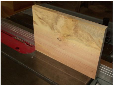
You should now have a nice rebate cut into the long side of the board. Repeat this process for the other short board measuring 30cm long by 21cm wide (11 13/16" long by 8 1/4" wide).
