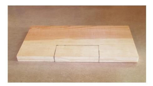
Now cut along the two 5cm (1 15/16") lines with a handsaw or table saw. Stop each cut at the end of the line. See the picture for details.
