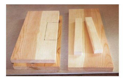
First we need to outline where our hive entrance will be. Take one of the floor halves measuring 33.5cm by 16.75cm (13 3/16" by 6 5/8") pieces and grab a ruler. Measuring from one edge of the board, mark the following points on the long side of the board:
