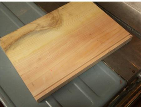
Now take the board and stand it upright. Place the previous cut towards the fence and run the board through the table saw.
