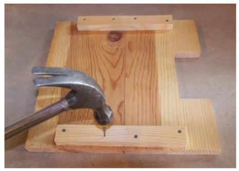
Now it is time to add the landing board. Rotate the fastened assembly 90 degrees and lay the 41cm by 16cm (16 1/8" by 6 5/16") board on the floor. Measure from one
