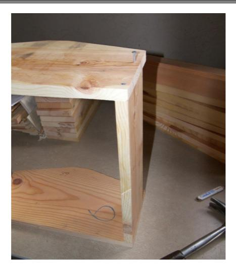
Take the cover board and lay it on the short sides of the box. It should just fit between the end gables of the longer sides. Fasten it in place.
