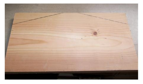
1/4" wide) and lay it on your work surface. Decide which long side of the board you want to be the top. Now place a mark on each side of the board 16cm (6 5/16") up from the bottom. If you have a combination square or speed square, set it for 72 degrees. Place the square at the mark and draw a line towards the top of the board
