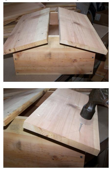
Take the ridge panel measuring 50cm long by 6cm wide (19 11/16" long by 2 3/8" wide) and lay it over the space between the roof panels. It will hang over a bit on each side. Align the ends of the ridge panel flush with the ends of the roof panels.
