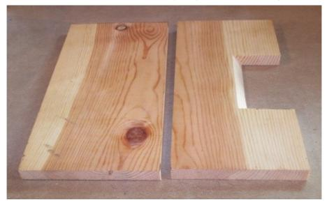
Butt the edges flush together and lay the two short pieces measuring 21cm by 3cm (8 1/4'' by 1 3/16'') pieces crossway over the two floor halves about 1 cm from the edge. Center each piece on the seam formed by the edges of the two larger boards. Fasten the wood together. Be sure to hold the assembly straight as you fasten it.
