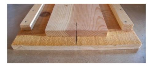
Now measure in from the edge of the floor about 1cm and make a mark with your pencil. Align the edge of the landing board with the mark. Add a fastener to hold the landing board in the center of the floor.
