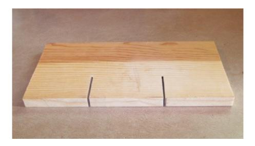
Take a chisel and remove the extra wood between the two cuts. When finished, you may want to use some sandpaper to smooth out the chiseled area.
