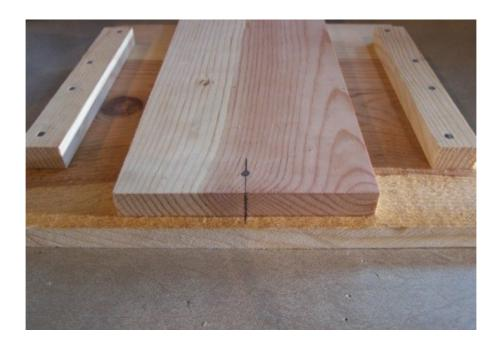
Now flip the floor assembly 180 degrees and measure the distance from each edge of the floor board to the side of the landing board. Nudge the landing board left or right until the distances on each side are equal. Use a fastener to hold the board in place.
